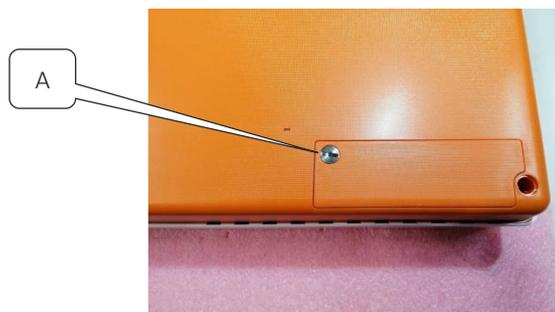
3. Disconnect the battery and remove it from the compartment:
