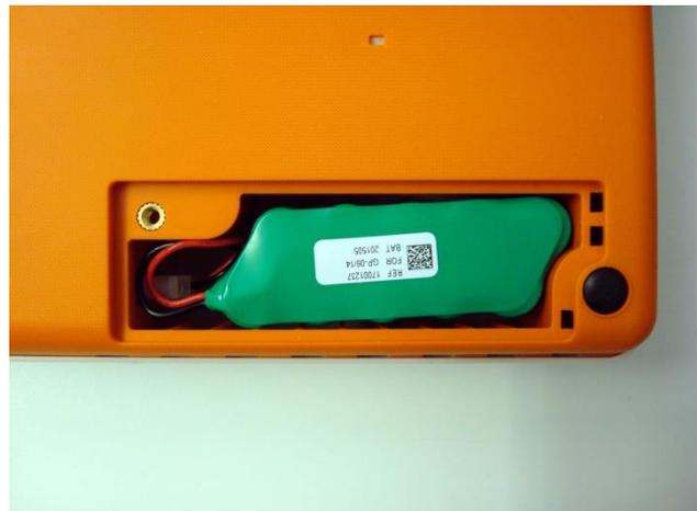
4. Place the battery in its compartment.
