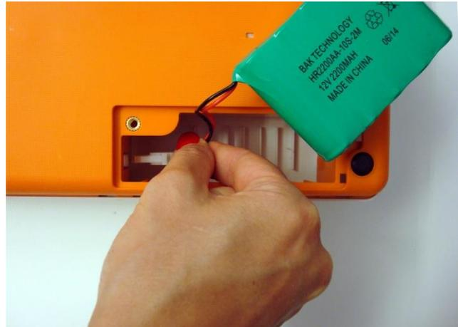
2. Disconnect the battery connector.
