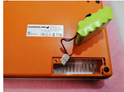
4. Leave the device with the battery disconnected for 60 minutes (the time required to reset the touchscreen calibration memory).
