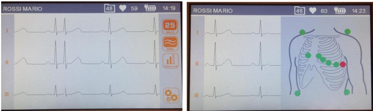
Display in real time and display in real time with Torso screen
